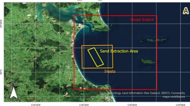
Figure 1: Map showing the proposed sand extraction area (yellow rectangle) and extents of the highest resolution wave model nest (red rectangle).
