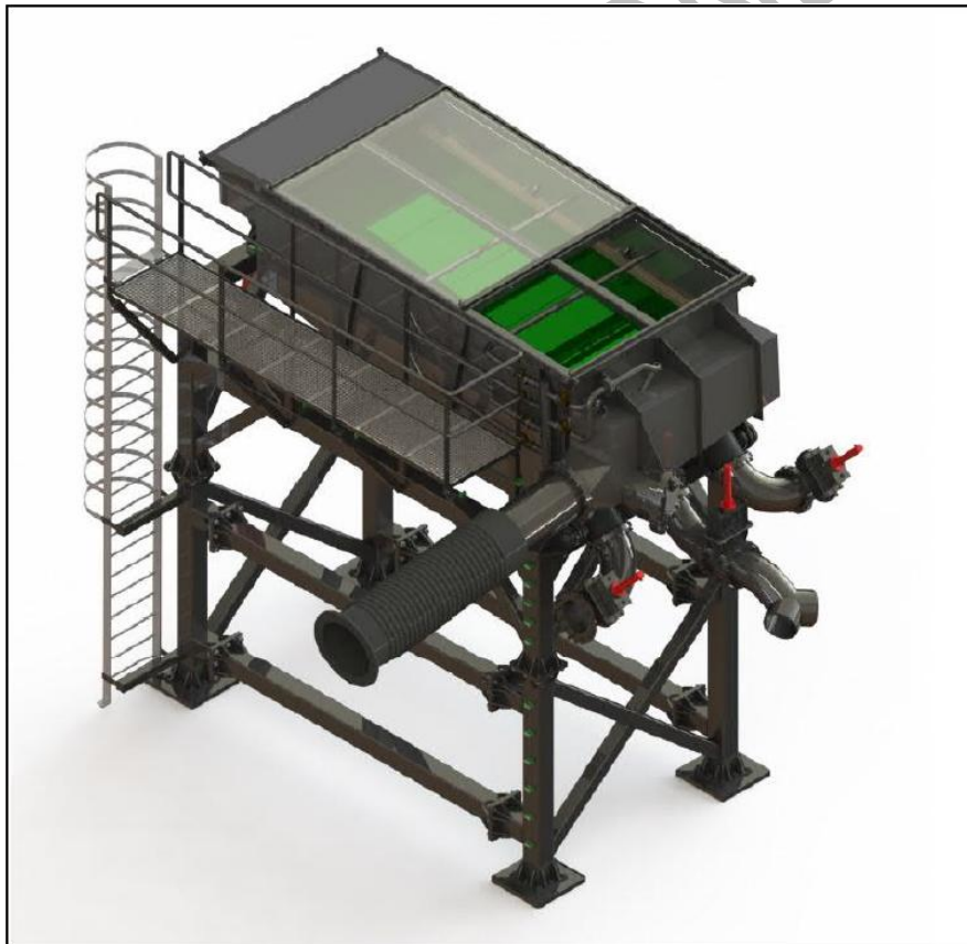
Figure 9: Plan of sand 'screening deck' on the William Fraser
